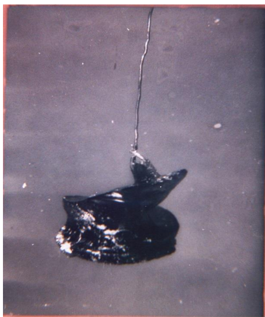
FIG.1A. Single crystal grown by cz technique.
